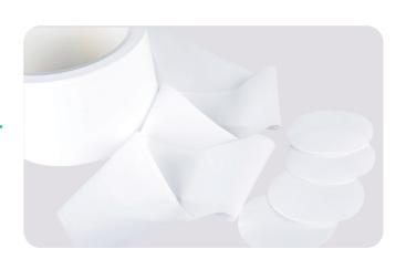
PTFE Membranes are self-supporting so backing liners are not required. Being naturally hydrophobic FLONTEX™100 is an excellent venting material & due to its non-stick quality, exhibits unrivalled filter cake release properties. As standard, our PTFE membranes are supplied as punched discs, however, semi-finished material in roll or sheet form is available on request.
